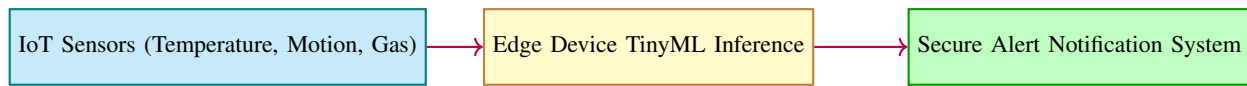
Fig. 4: Layered architecture of the proposed secure TinyML-driven emergency detection system operating at the network edge.
